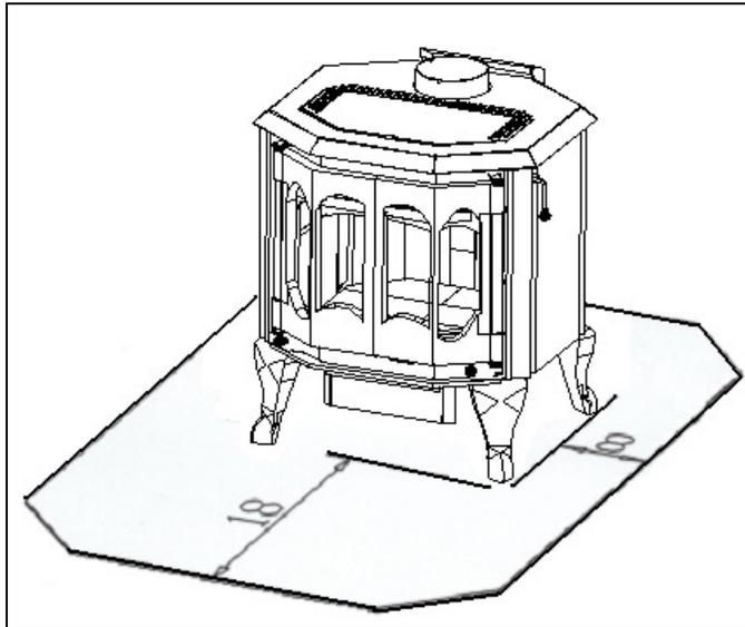
You must install a fireproof plate under the appliance, which must exceed it of 18 inches at the front, of 8 inches at the sides and of 8 inches at the back.
