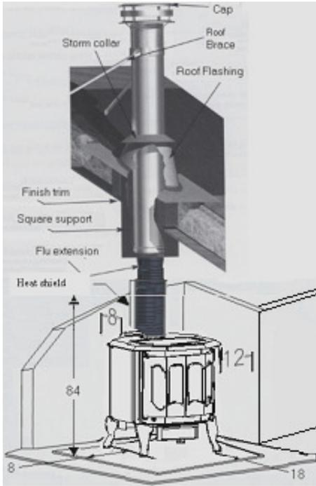
The *Mystere* wood appliance must be installed in accordance with the applicable local laws or the CAN/CSA-B365, NFPA211 ( USA ) norms. Install the chimney following the manufacturer's instructions.
