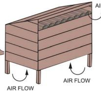
Cut the wood so that it will fit horizontally, front to back, making for easier loading and less of a likelihood that the wood will roll onto the glass.
