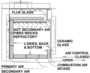
sides and back are shielded to direct the heat upwards and forwards into the room.
