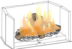
A flash fire is a small fire burned quickly when you don't need much heat. After your kindling has "caught", load at least 3 pieces of wood, stacked loosely. Burn with the draft control fully open or closed only slightly.
