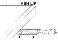
Adjusting the air control regulates the temperature. The draft can be adjusted from a low burn rate with the handle in fully, to a fast burn rate with the handle fully out.
