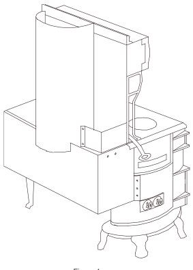
Figure 4 Illustration of Oval with heat shield kit
