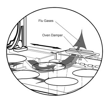
Figure 9 - shows oven damper open
