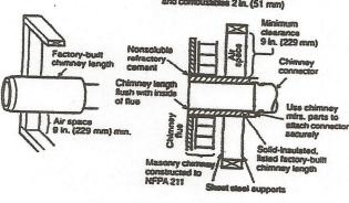
Solid-insulated, listed factory-built chimney length of the same inside diameter as the chimney connector and having 1 in. (25.4 mm) or more of insulation with a minimum 9-in. (229-mm) air space between the outer wall of the chimney length and combustibles
