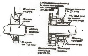
Solid-insulated, listed factory-built chimney length with an inside diameter 2 in. (51 mm) larger than the chimney connector and having 1 in. (25 mm) or more of insulation, serving as a pass-through for a single wall sheet steel chimney connector of minimum 24 gauge (0.024 in. (0.61 mm)) thickness, with a minimum 2-tin. (51-mm) air space between the outer wall of chimney section and combustibles.
